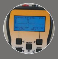
The rapidtrace stores up to 50 traces at one time and records the time and date of each trace performed
