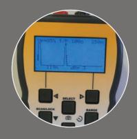
Here we can see the gain control to provide a clearer view of the trace
