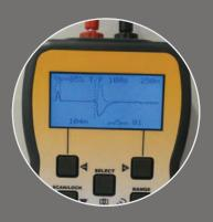
The trace comparison feature allows users to compare saved traces with a live trace
