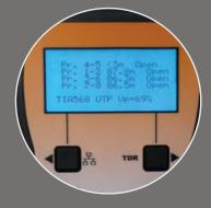
The RapidTrace 700's TDR functionality allows users to accurately identify fault types and exact distance on each pair of a specific cable
