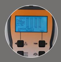
The wiremap test gives a clear indication of any wiring faults and certifies the cable continuity.
